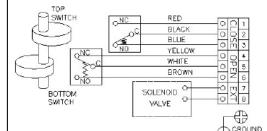
Standard switch: 2 x Omron SPDT SS5GL AC: 250V 3A, 125V 5A DC: 30V 4A
