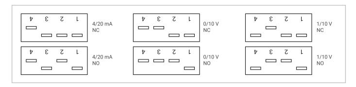
Configurations set up by using DIPs, should have the same Input and Output Signal.
