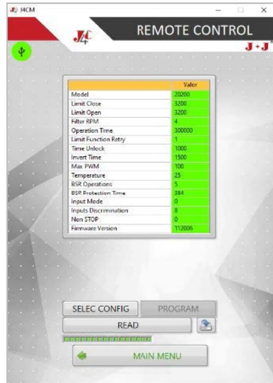
If you click on **PARAMETERS**, the following screen will open, showing the actuator parameters, loaded during the mass production process.
