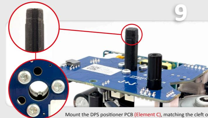
Mount the DPS positioner PCB (Element C), matching the cleft of the shaft with the key inside the DPS gear.
