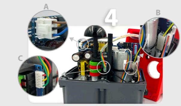
Remove the cables (from the cover) connected to the actuator PCB (Fig. A, B and C).
