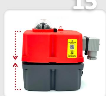
Carefully mount the cover, minding the cables not to be pressed.
