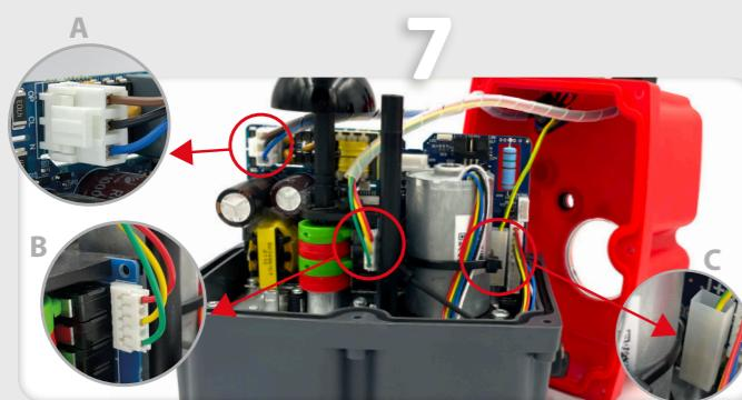
Take the DPS cover (Element A) and connect its cables, following (Fig. A, B, C).
